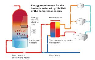
The compressor cooling system can be modified to provide water at around 80°C to pre-heat the customers own feed water to their heating systems (water or steam) and thus reduce their energy load through the water/steam heater. Savings are typically 22–30% of the compressor motor rating kW.
